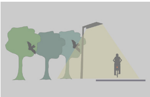
Figure 5.4. Avoidance of light trespass by installing shielded luminaries. Left – conventional luminaire with light spillage into the adjacent forest habitat, right – shielded luminaire that focuses the light cone only on the area where it is needed (© H. LIMPENS).
