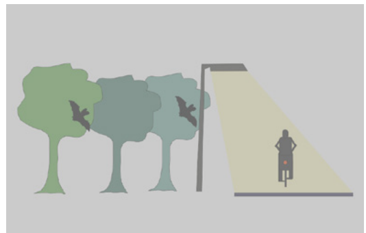
Figure 5.4. Avoidance of light trespass by installing shielded luminaries. Left – conventional luminaire with light spillage into the adjacent forest habitat, right – shielded luminaire that focuses the light cone only on the area where it is needed (© H. LIMPENS).
